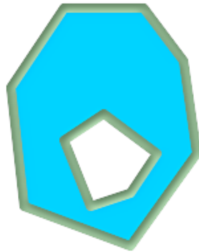
polygon holes with boundary multilinestring
