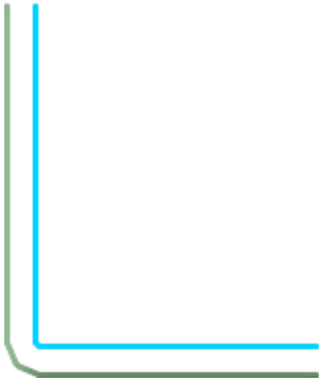
15, 'quad_segs=4 join=bevel' shown with original line
