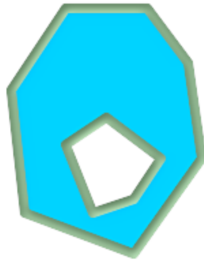
polygon holes with boundary multilinestring
